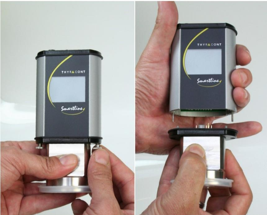
Now attach the replacement sensor (3) to the electronics unit (5). Take care of a correct fit of the profiled sealing (4) at the housing cover. Tighten the knurled nuts (1) again, mind the sealing washers (2).
