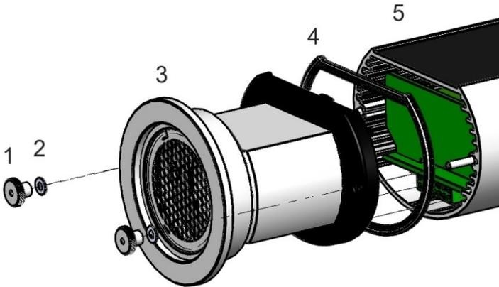
Unscrew the two knurled nuts (1) at the bottom cover of the transducer as shown below and pull the electronics unit (5) straight and without twisting off the sensor (3). Pay attention to the sealing washers (2).
