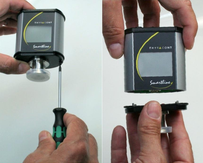
Now attach the replacement sensor to the electronics unit. Take care of a correct fit of the profiled sealing at the housing cover. Fix the sensor by tightening the Torx screws again.
