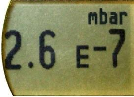
In order to change the display unit (mbar, Torr, hPa) hold the »Adj« key pressed while connecting power supply until the display shows »Unit«. Then select the desired unit by pressing the »Adj« key. After 5 seconds without further keypress the setting is saved!
